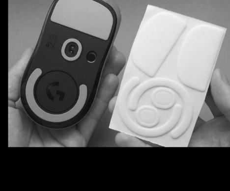
removed completely and carefully using a flat tool (e.g. plastic spatula). Avoid damage and scratches.
